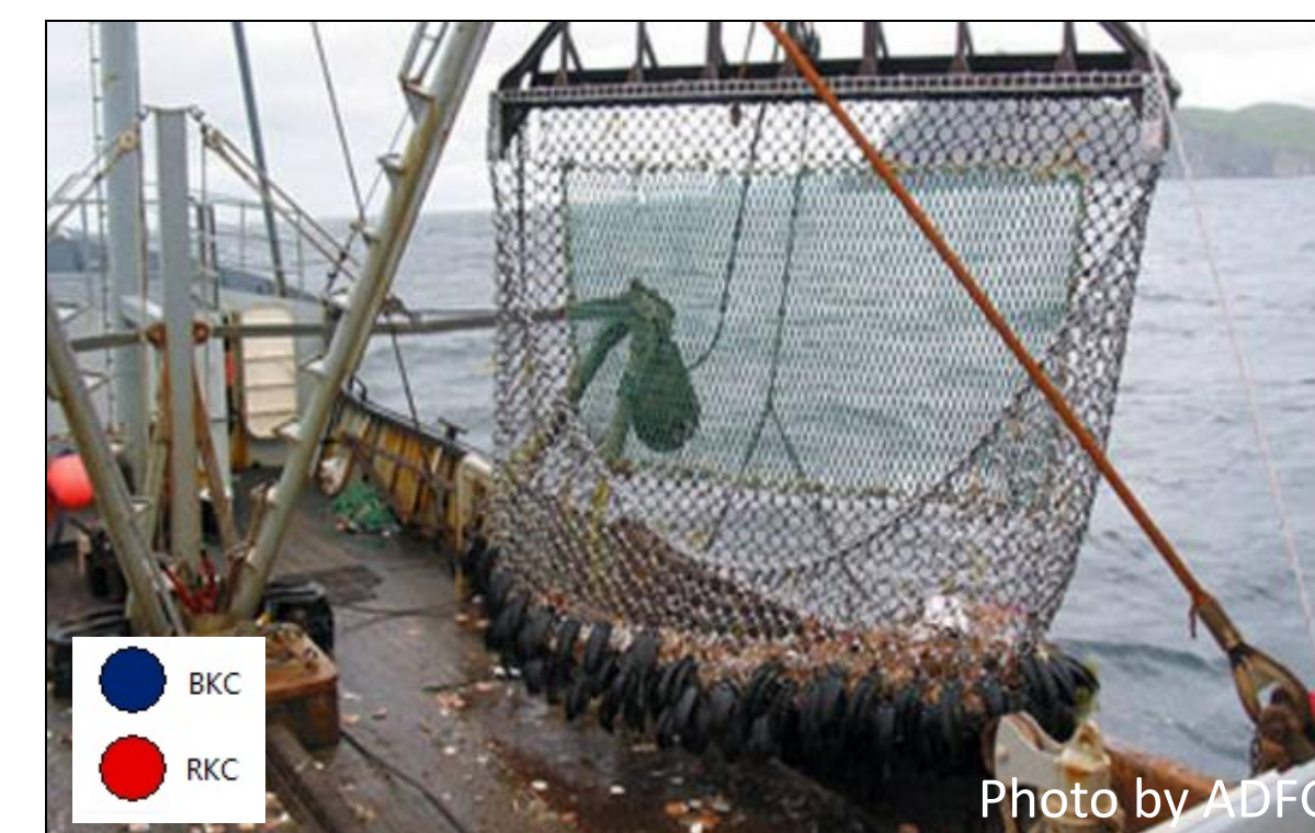
Fig. 3) An example of a Rock Dredge type bottom trawl net used in 1983-84 study to quantify crab and assess bottom habitat.
