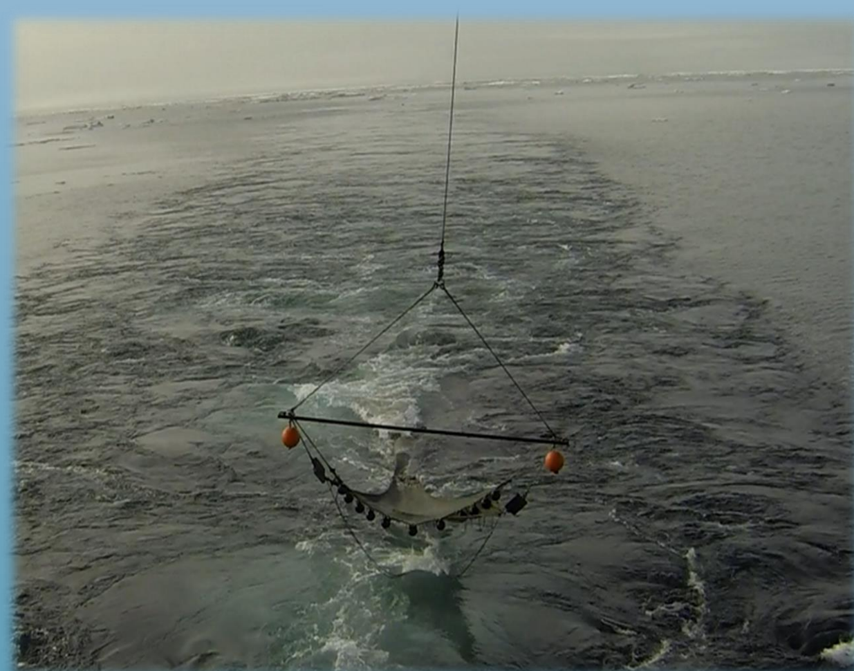
Fig 1: Plumb staff beam trawl deployed from the USCGC Healy.
