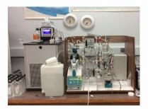
OARC operates MARIANDA instruments to quantify dissolved inorganic carbon (DIC) and total alkalinity (TA). DIC is measured using the lab's AIRICA instrument, while TA is measured on a VINDTA.
