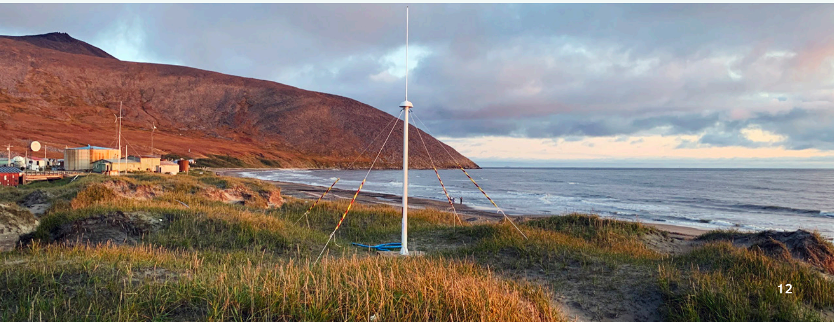
▼ HF radar antennas installed in Wales measure ocean currents in the Bering Strait. Photo by Hank Statscewich.
