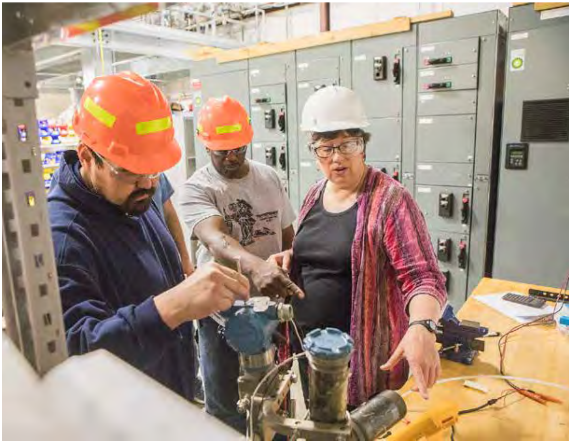
Students Glen Morgan, left, and Ernest Holt, center, listen as Teresa Lantz, assistant professor of process technology, demonstrates how to use a bubbler to monitor water levels in a tank in July 2017. Morgan and Holt were participating in the UAF Community and Technical College's mining mill operator training program at a facility leased from the Fairbanks Pipeline Training Center off Van Horn Road.
