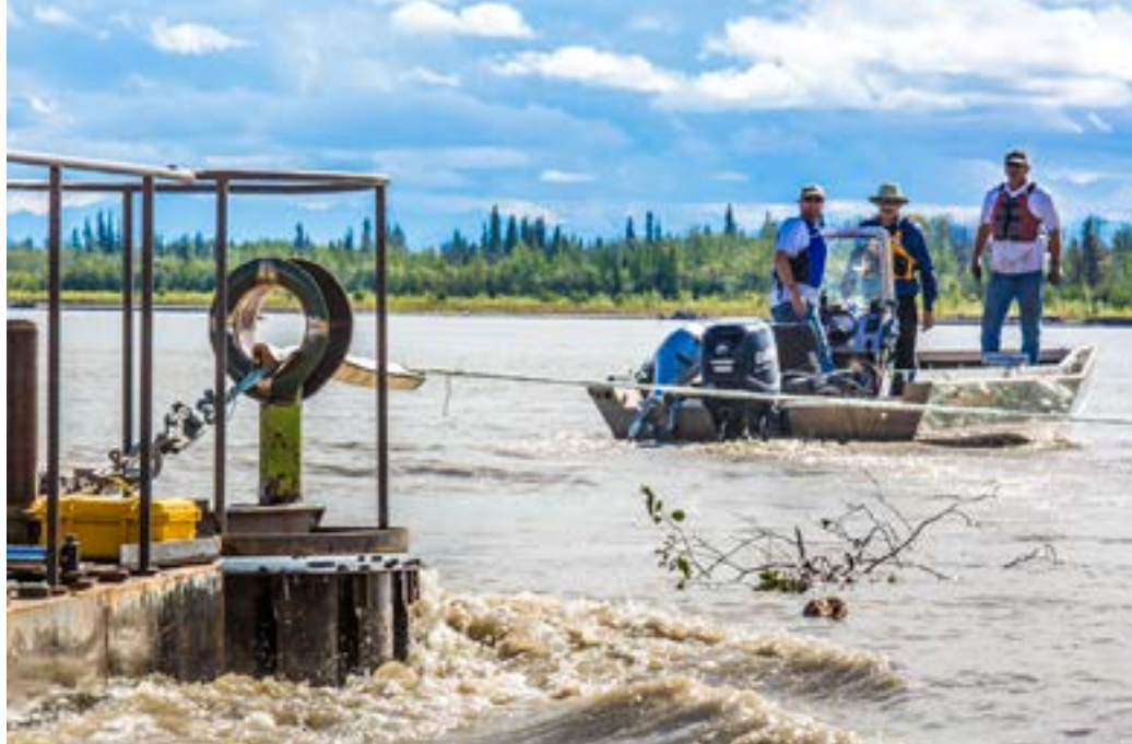
Staff test the efficacy of the debris diverter by tossing branches into the Tanana River in August 2012.
